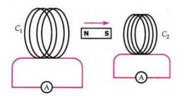
$C_1$  and  $C_2$  as shown in Fig. What will be the direction of induced current in each coil as seen from the magnet ? Justify your answer.
