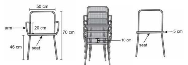
The dimensions of the seat (in cm) is  $50 \times 40 \times 5$ .
