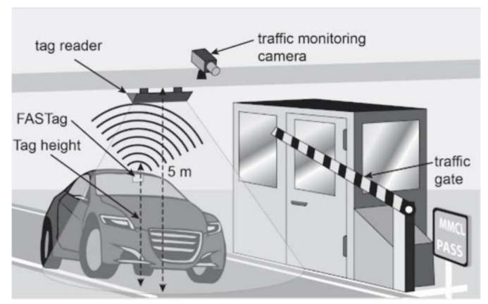
For the tag scanner to function properly the speed of a car needs to be less than 30 km per hour. A car with a tag installed at a height of 1.5 m from the ground enters the scanner zone.
